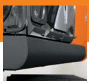
■ Reinforced D-channel side frames provide maximum cab and component protection.
