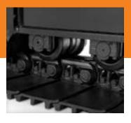
■ With large idlers, rollers, and strutted links, the sealed and lubricated undercarriage delivers long, reliable performance.
