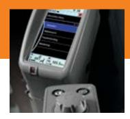
Multi-language LCD monitor and rotary dial provide access to a wealth of info and functions. Just turn and tap to select work modes, check diagnostic codes, monitor maintenance intervals, set cab temperature, and make simple attachment hydraulic-flow adjustments, plus more.
