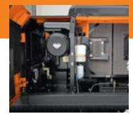
Hinged service doors provide wide-open access to cooler cores for simplified debris clean-out.
